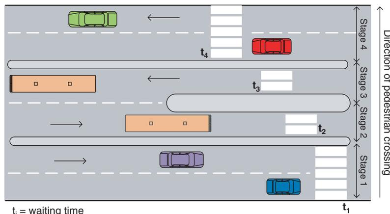
FIGURE 3 Schematic drawing of crossing.
